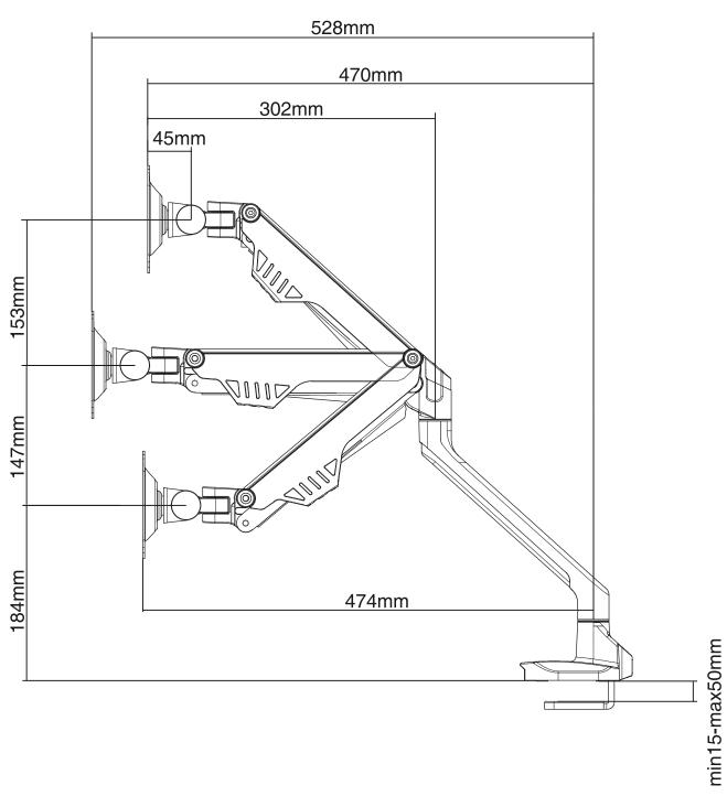
Neomounts Measuring unit: mm
